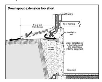
The rule of thumb to apply is a 4 to 6 feet extension away from the home for downspouts, and also good sloped grading of the landscaping away from the home, to prevent water from pooling and potentially causing damage to the foundation.
